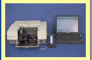
Thermo Scientific FT-IR spectrometer with PAC 300 Photoacoustic E.S.P. accessory installed
